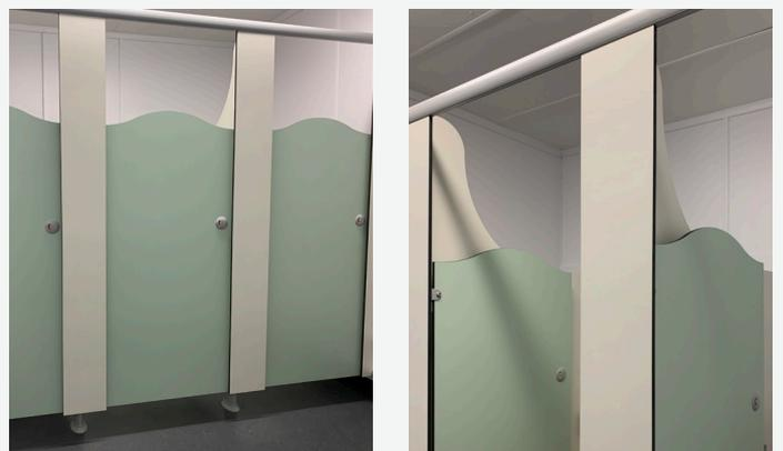
With 1300mm high cubicle doors and shaped partitions, staff will be able to supervise students when required. The anti-finger trap hinges and emergency release indicator bolts that come as standard, made Genesis an ideal cubicle choice.
